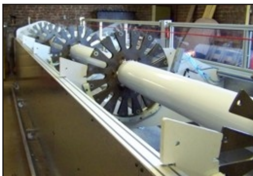
Photo of the 13 metre long tube drilling machine
